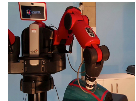
Figure 2 Baxter robot sweeping the test surface.
