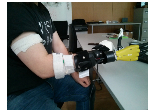
Figure 1. Subject wearing the prosthetic hand and the sensors on his forearm. The sensors are secured with an elastic bandage.
